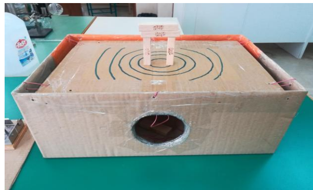
Figure 3. Assembled simulator showing the rear access hole and a three-block tower placed at the epicentre (Source: Authors' own elaboration)
