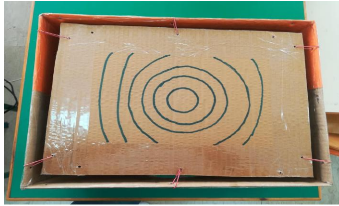
Figure 2. Top view of the assembled simulator. The cardboard platform is suspended inside the paper box by rubber bands, allowing it to oscillate during the simulated earthquake (Source: Authors' own elaboration)
