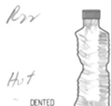
Figure 11. Hot denting bottle (R22) (Source: Authors' own elaboration)
