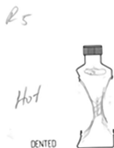
Figure 10. Hot denting bottle (R5) (Source: Authors' own elaboration)
