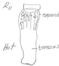
Figure 5. Hot denting bottle (R11) (Source: Authors' own elaboration)
