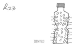
Figure 8. Hot denting bottle (R23) (Source: Authors' own elaboration)
