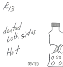
Figure 6. Hot denting bottle (R13) (Source: Authors' own elaboration)
